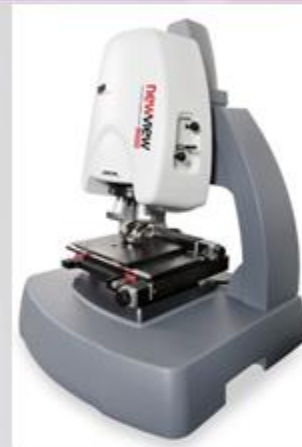
White light interferometry (Zygo NewView™)
