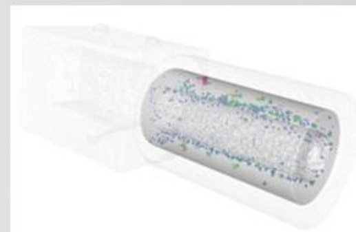
Sub-surface porosity analyses
